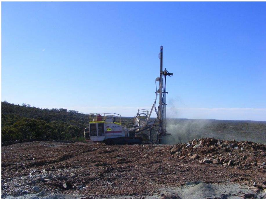
**Image 2.** Production drilling at Pit 1
